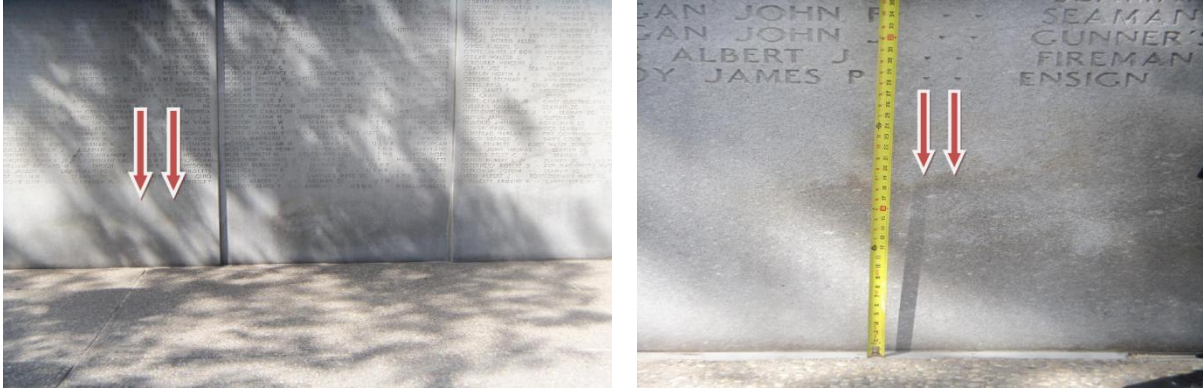
Figure 4. High water mark at East Coast Memorial in Manhattan. The high water mark indicates a flood of 1.6 ft.
