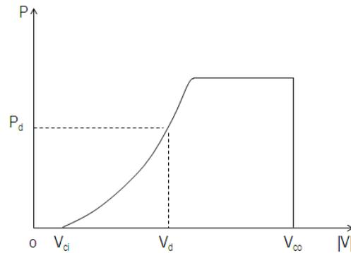
**Figure 7. Power curve of MHK energy generation system.  $P_d$  is the designed minimum power output of the system, and  $V_d$  is the corresponding current velocity.**
