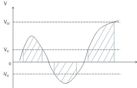
**Figure 6. Current velocity history. The shadow area indicates MHK energy available for a turbine to generate power.**
