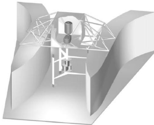
**Figure 5. A designed and tested argumentation channel for a floating MHK turbine (from Ponta and Jacovkis, 2008).**
