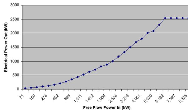
**Figure 4. Power curve of Marine current turbine (from Bedard, 2005).**
