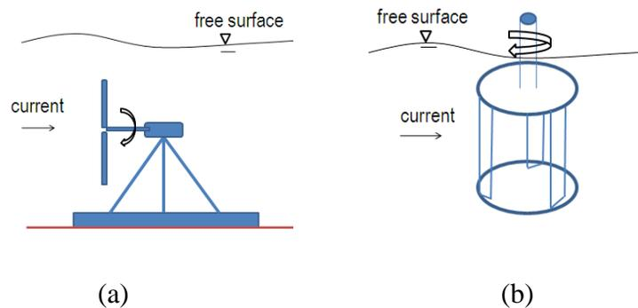
**Figure 2. Categories of MHK energy turbines. a) Horizontal axis turbines. b) Vertical axis turbines.**
