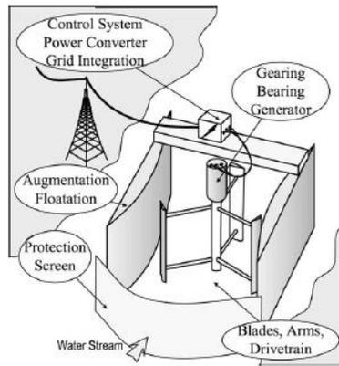
**Figure 1. Schematic representation of power generation using MHK energy (from Khan et al., 2009).**
